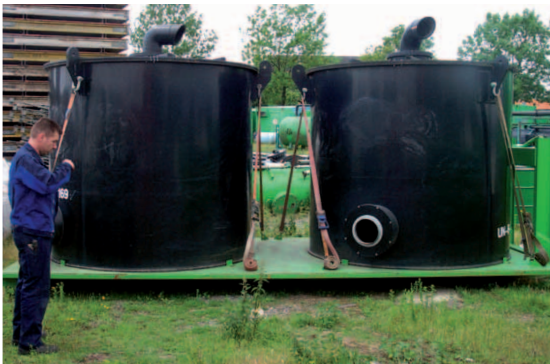
2 LAK 5.000 activated carbon filters fixed on a plate for fast application and replacement
